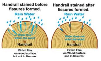
We strongly recommend that handrail be allowed to dry to less than 20% moisture content before doing anything to them. This may take two to six months depending on how green they are and the diameter of the rails.
